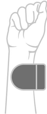
The hands free pulls should be installed with the opening part towards the leading edge of the door.
